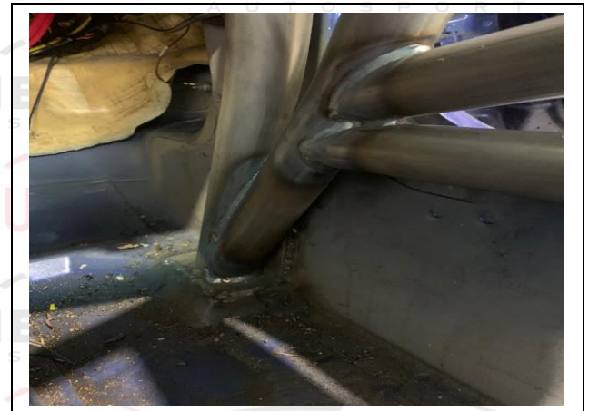
PHOTO 6 FRONT ROLLBAR TO FLOOR ATTACHMENT
