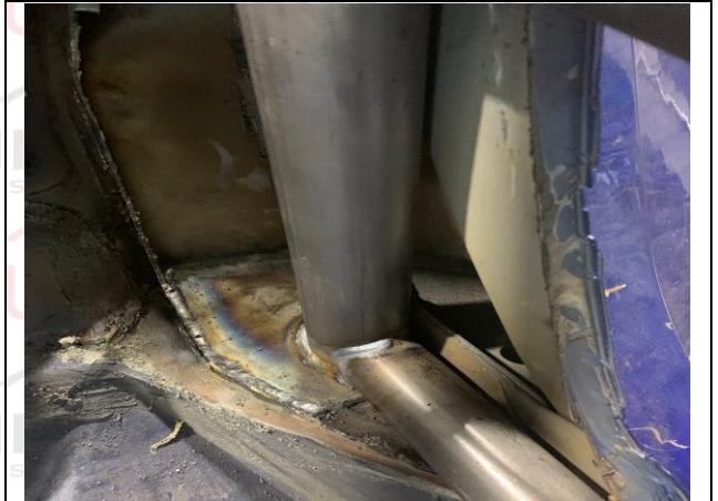
PHOTO 4 MAIN ROLLBAR TO FLOOR ATTACHMENT
